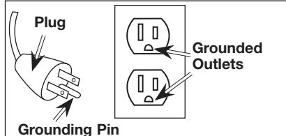
3. Inspect the plug and cord before each use. Do not use if there are signs of damage.
